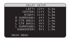
The DELAY SETUP menu, which is reached from the MAIN menu, allows you to set the delay for individual speakers. This ensures that the sound from each speaker arrives simultaneously at the listening position, even when the speakers are not all placed at equal distances from the listener. Increase the delay to speakers located closer to the seating area and decrease the delay to speakers located farther from the seating area.
